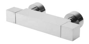
Factor bottom outlet bar valve - single function 265(w) x 40 x 106mm(d) Minimum pressure 0.1bar
