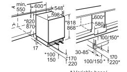
\* Variable base/ substructure height Space for electrical connection next to the appliance on the left or right-hand side. Ventilation space in the base.
