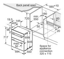
If the appliance will be installed underneath a hob, the following worktop thicknesses (including substructure if necessary) must be taken into account.
