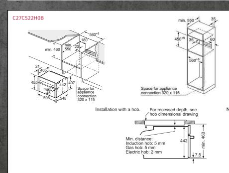
Measurements in mm. The line drawings featured in this brochure are provided as a guide to general dimer For full dimensional and installation details please refer to the documentation supplied with the appliance.
