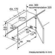
min. 300 ation 320 dia. 170 measurements in mm
