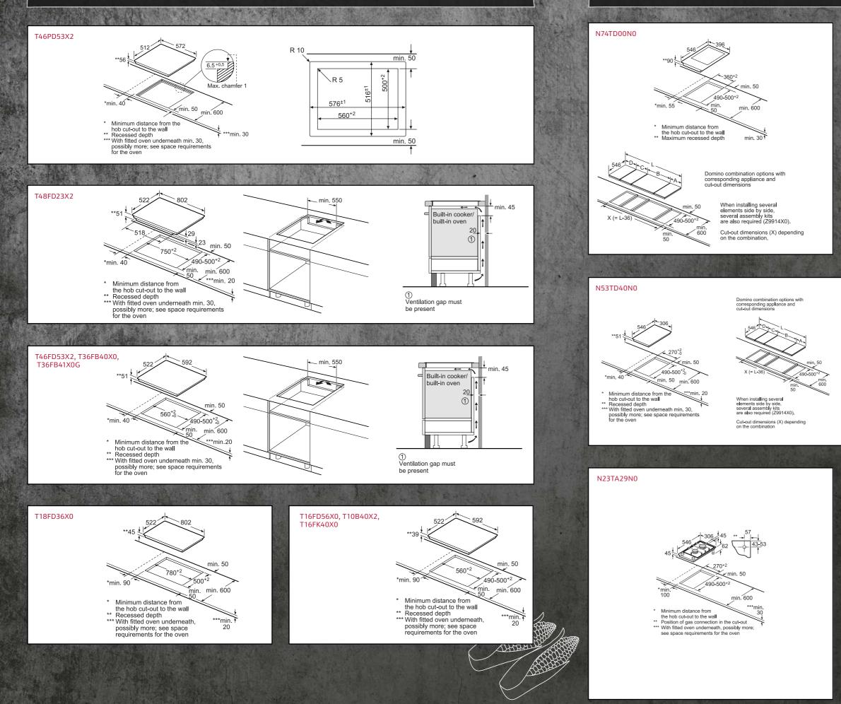
18 Measurements in mm. The line drawings featured in this brochure are provided as a guide to general dimensions only and are subject to amendment without prior notice. For full dimensional and installation details please refer to the documentation supplied with the appliance.
