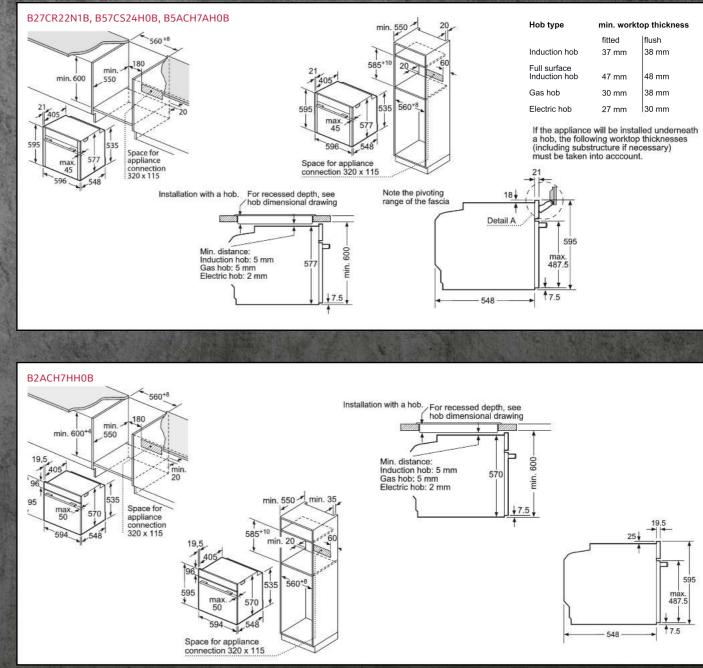
Measurements in mm. The line drawings featured in this brochure are provided as a guide to general dimer For full dimensional and installation details please refer to the documentation supplied with the appliance.
