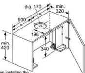
When installing the 90 cm telescopic hood in a 90 cm wide wall-hanging cupboard, the mounting kit is required. The two mounting brackets are screwed onto the right and left of the kitchen unit. Installation in accordance with template. measurements in mm
