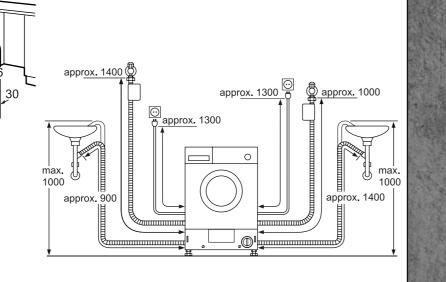
If, after fitting, the HydroSafe inlet hose to the installation is not long enough, it can be lengthened with the connecting kit WZ 10130 (length 2.5 m). W7460X5GB 1063 598 -632-848 - 590-
